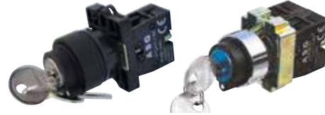
ANAHTARLI BUTON 3A / 240 V AC, IP 44
