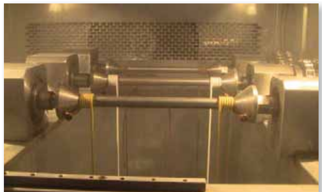
Cable samples in a cyclic strength test.
