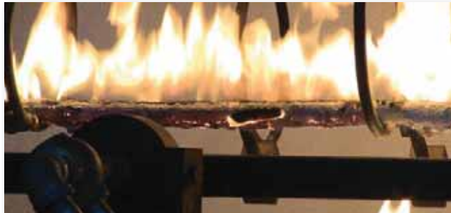
The tested cable should be able to carry voltage for 3 hours.
