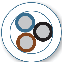
Outer sheath wall thickness cross-sectional view.
