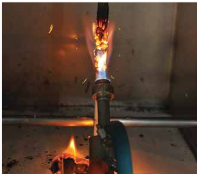
An improper cable sample in a burning droplet test.
